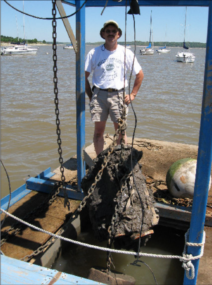
Photo #1: Daryl Strouts next to an old truck engine used on early moorings
